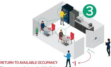
Once max capacity is reached, the first exit registered by a door contact opened from within will restore occupancy count to below capacity.
